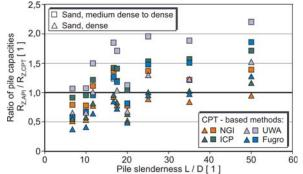
Fig. 3 Comparison of tensile pile capacities in sand soil according to the usual approach (API) and according to recently developed method
