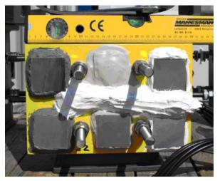
Fig. 2 Test coupon with online monitoring
